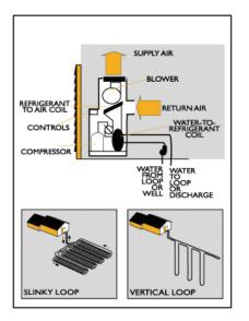
A water/anti-freeze solution circulates in underground piping transferring heat to and from the heat pump.
