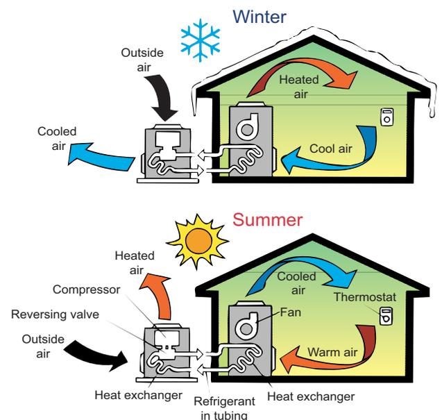
When in the heating mode, the outdoor condenser can be continuously controlled during peak demand periods, monthly billing peak periods, or system emergencies for up to a maximum of 12 hours per day, and 400 hours total per heating season.
